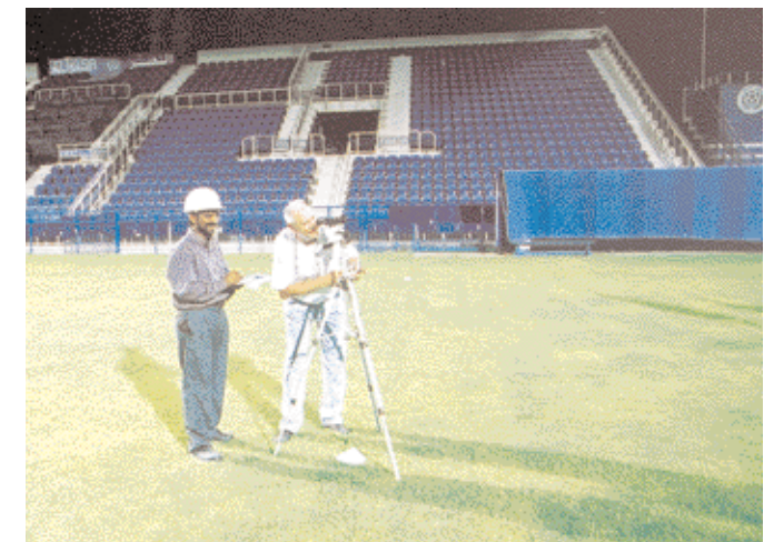
FIGURE 5-1-Fbis: Measuring of vertical (camera) illuminance.
