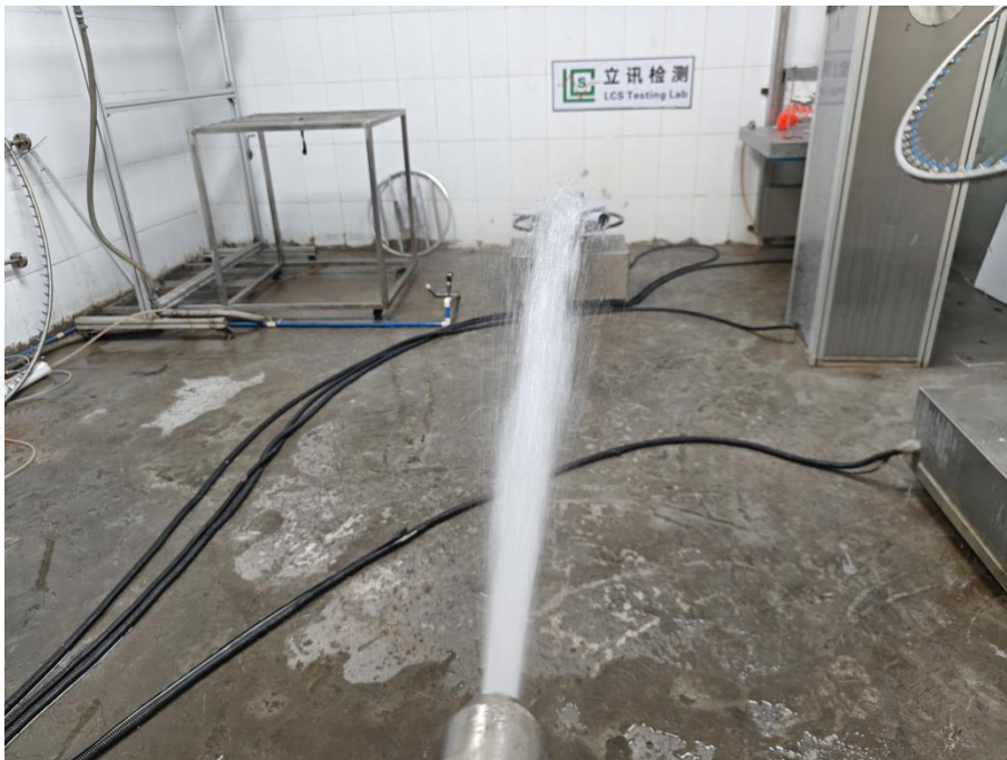
Photo 4: IPX6 test of model MSL-F240
