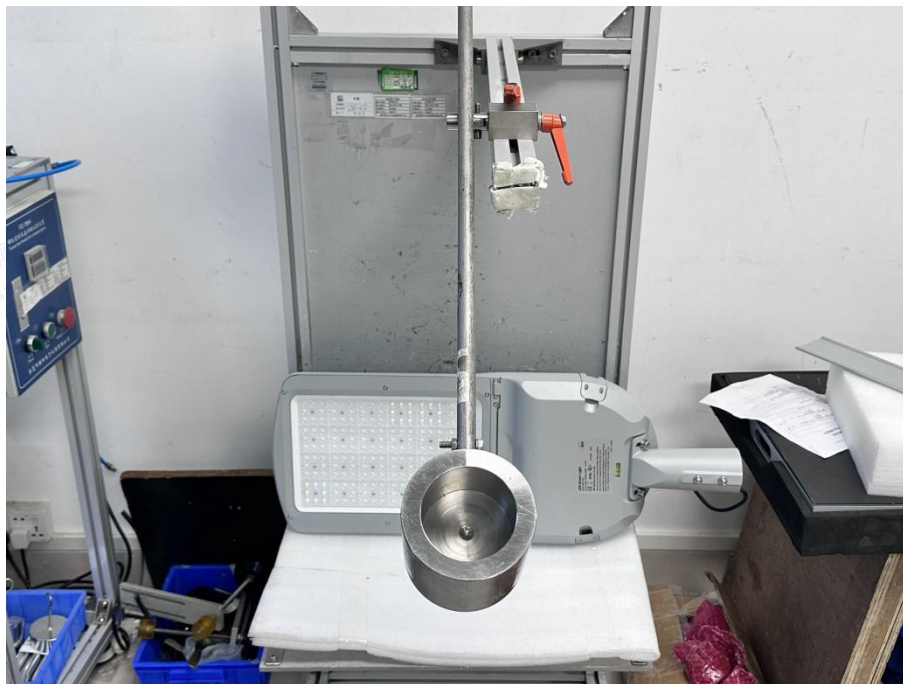
Photo 3: IK10 test of model MSL-F240
