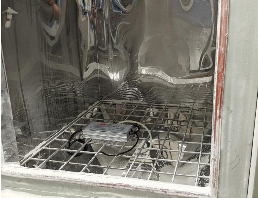
Photo 3: IP6X test of model X6-320M062
