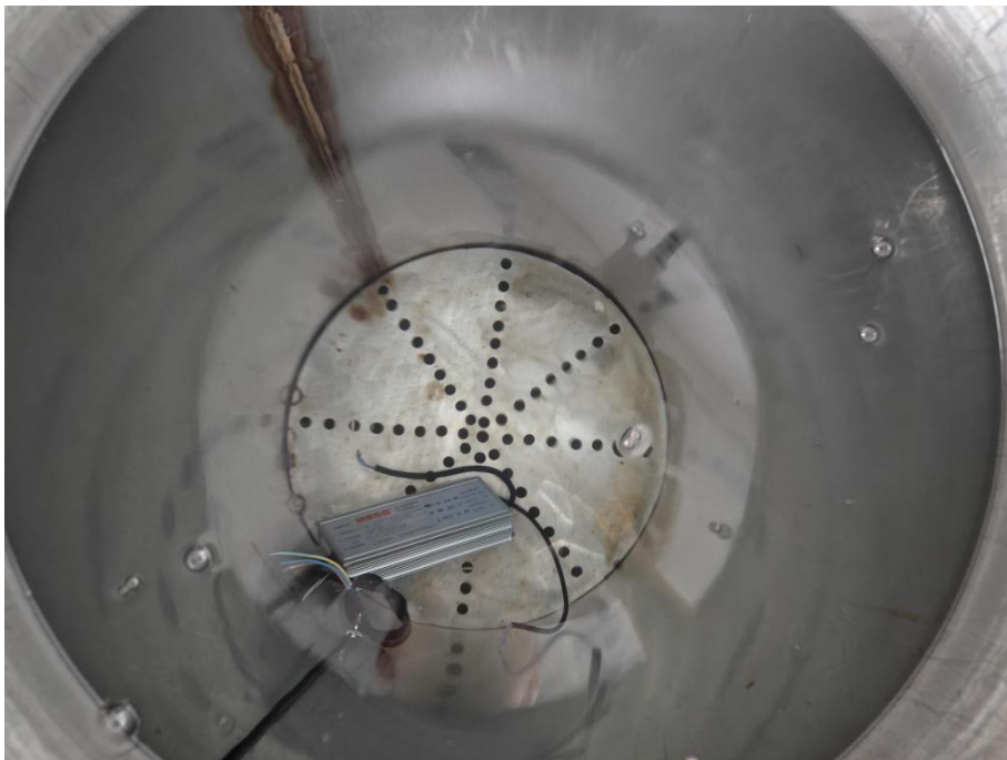
Photo 4: IPX7 test of model X6-320M062
