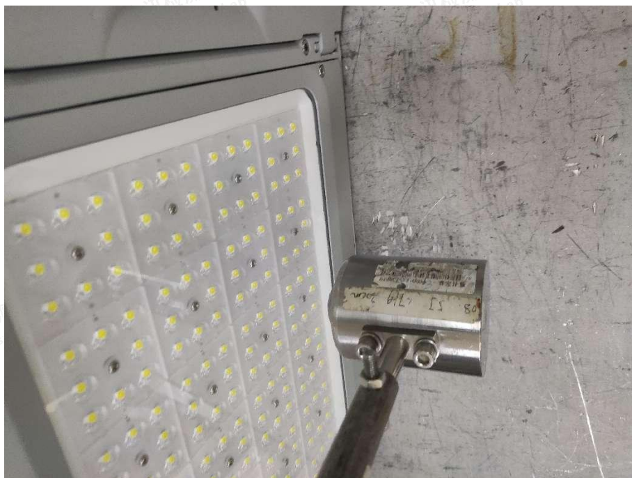
Photo 4: IK08 test of model MSL-F300
