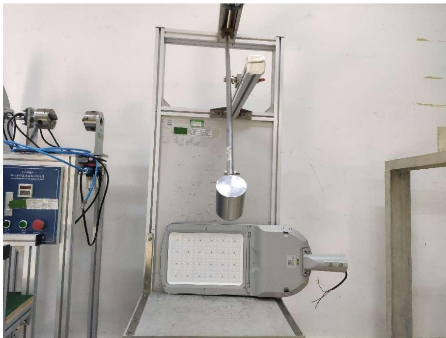
Photo 3: IK08 test of model MSL-F300
