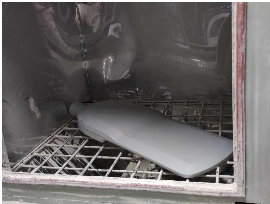
Photo 3: IP6X test of model MSL-F300
