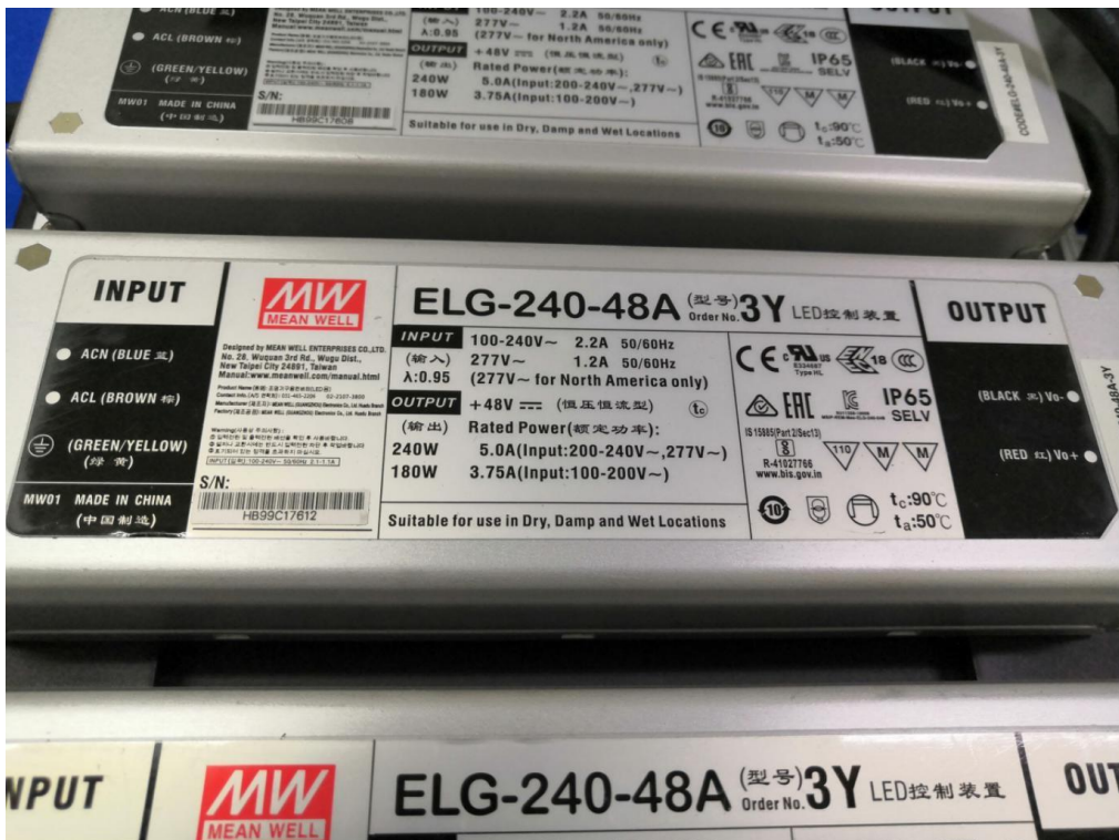
Figure 6: LED driver of model ELG-240-48A
