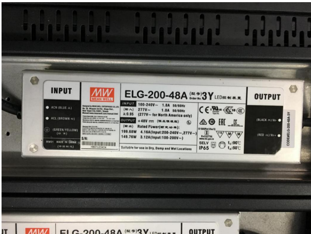
Figure 8: LED driver of model ELG-200-48A
