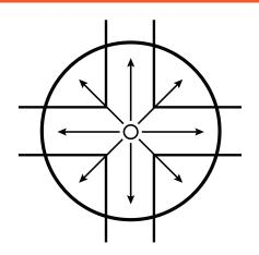
The Type V distribution produces a circular distribution that has the same intensity at all angles. This distribution has a circular symmetry of candlepower that is essentially the same at all lateral angles. It is intended for luminaire mounting at or near center of roadways, center islands of parkway, and intersections. It is also meant for large, commercial parking lot lighting as well as areas where sufficient, evenly distributed light is necessary.
